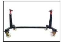
The **B4000HB / B6000HB** boat dollies has a heavy duty steel design allowing it to not be damaged under a heavy load. Total holding capacity of 4000/6000 kg per pair these dollies make able to support most boats. Our removable pins make adjusting this dolly to fit your boat a simple process.
